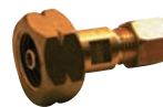
GT120 Tank connector for remote gas regulator (GT2005-2) with 1/2" left hand female thread inlet & 8mm olive outlet for copper pipe.
