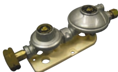
GT2005-1 LPG regulator 30mbar for direct connection to gas tank with 1/2" left hand female thread inlet & 8mm olive outlet for copper pipe.
