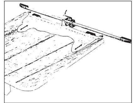
The hook n' lock is designed to firmly fix table to sidewall, while allowing lateral movement when unlocked, to make access to bed boxes easier, simply press down on central lock arm to release lock and slide table away without disturbing items on top of the table. Designed to complement our swing n' lock folding table leg to make up table. Securely anchors table for traveling and use while allowing the flexibility of position.
